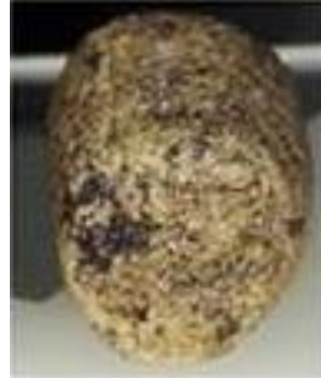
Consumed permanganate wax cylinder
